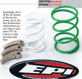
couldn't find a downside to the kit. We tested the RZR on an old asphalt service road (for traction consistency) loaded down with passengers. With the stock clutching, our RZR would hit the 70-yard mark in 4.9 seconds very consistently. Believe it or not, the same RZR on the same run, with the same passengers would hit the same 70-yard mark in 4.4 seconds. That half-second difference in acceleration time backs up the seat-of-the-pants feel.
